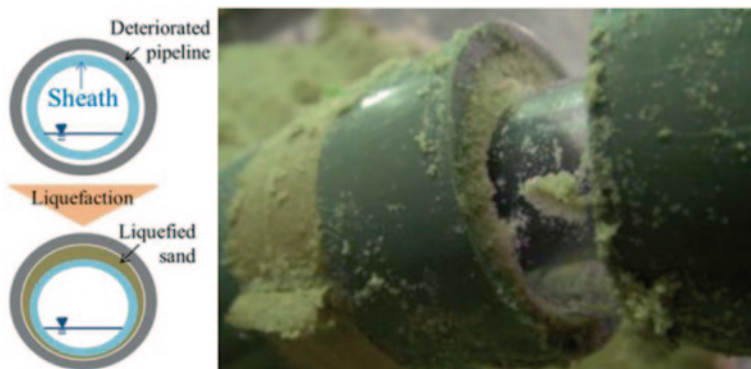
Fig. 46 Joints disconnection of buried pipelines and sheath pipe in it
