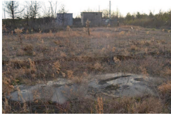
Fig. 14 Sand boils observed near IBRH20 recording instruments (background). Photo courtesy of R.W. Boulanger
