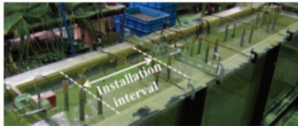
Fig. 19 Preparation of experiments with drainage pipes
