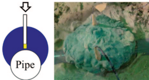
Fig. 27 Example of injection method and products (Grout.2~3 cases)
